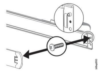
**Note:** This step is required for preventing non-operating transportation shock and vibration.
