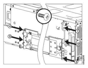
The (\*) screws in the rack-post diagram above are used for shipping and transport only. Each chassis thumbscrew and lower front rail screw secure the handle to the rack post. For more information, see the enclosure installation instructions in the *Hardware Installation* and *Maintenance Guide - Model 106*.
