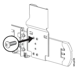
2. Attach 'C' bracket from rail kit to chassis with two screws (Item 1 under Table 1 on page 1) M4x4 PH. Torque: 12 lbf-in.
